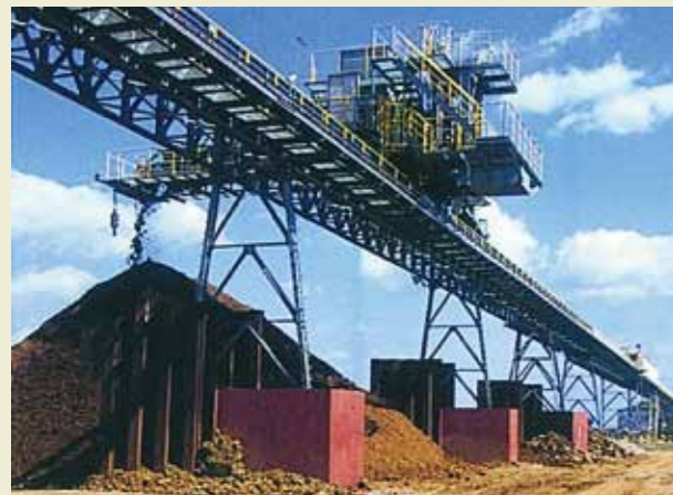
Ore Conveyor: The ore that has been unloaded is transported via 2.4 km long conveyor to the plant.
