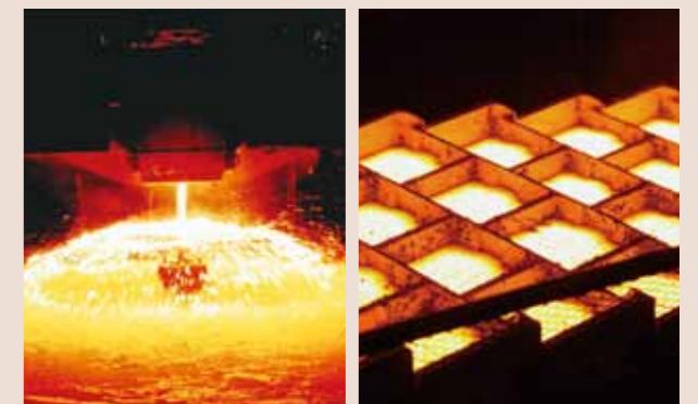
Shot casting: Molten metal is rapidly cooled with water in a water tank and finished into small particles.
