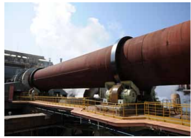
Rotary kiln: A calcining equipment, over 100m in total length that thermally processes dried ore by heating it to approximately 1,000 degrees Celsius.
