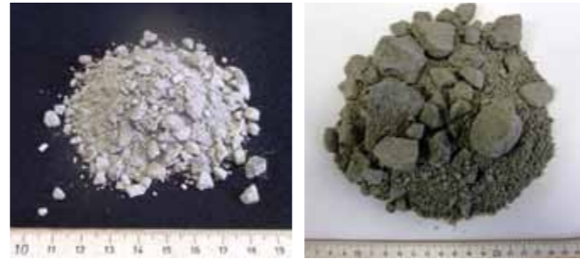
Ferronickel slag of 5 mm or less
