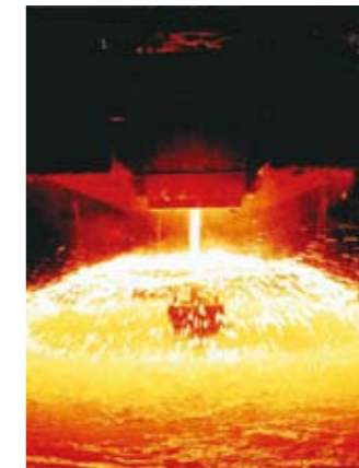
Shot casting: Molten metal is rapidly cooled with water in a water tank and finished into small particles.
