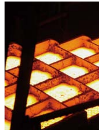
Ingot casting: Molten metal is poured into molds and finished into 20 kg ingots.
