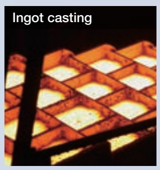
Molten metal is poured into molds and finished into 20kg ingots.
