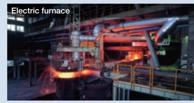
These are the world's largest electric furnaces that is heated by using electric resistance, and used for smelting ferronickel from ore.
