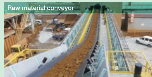
Raw material conveyor is total around 2.4km length.
