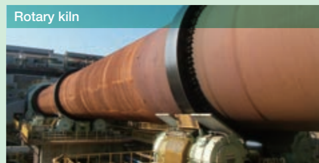
A calcining equipment, over 100m in total length that thermally processes dried ore by heating it to approximately 1,000 degrees Celsius.
