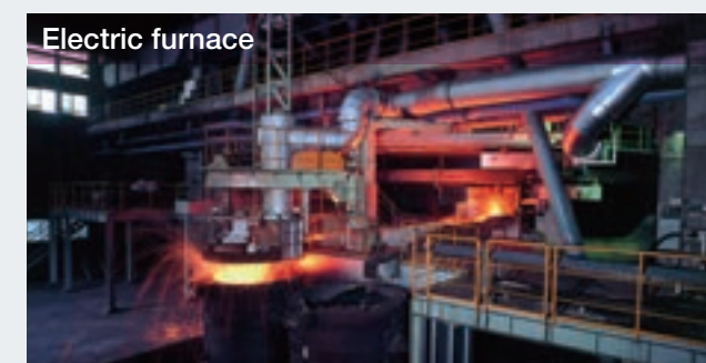
Electric furnace These are the world's largest electric furnaces that is heated by using electric resistance, and used for smelting ferronickel from ore.
