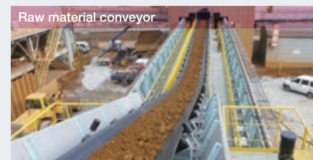
Raw material conveyor Conveyors totaling 2.4 km in length transport unloaded ore and other materials to the plant.
