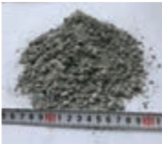
Ferronickel slag, 5mm or less
