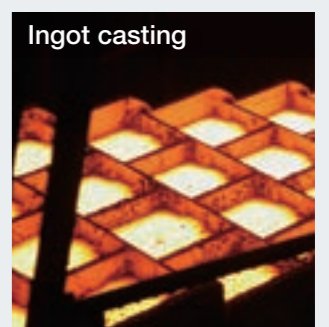
Ingot casting Molten metal is poured into molds and finished into 20kg ingots.
