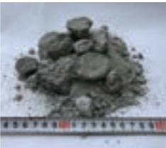
Ferronickel slag of 0 to 40mm
