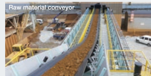
Raw material conveyor Conveyors totaling 2.4 km in length transport unloaded ore and other materials to the plant.
