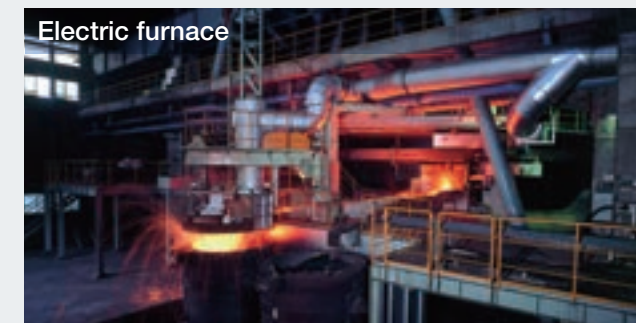
Electric furnace These are the world's largest electric furnaces that is heated by using electric resistance, and used for smelting ferronickel from ore.
